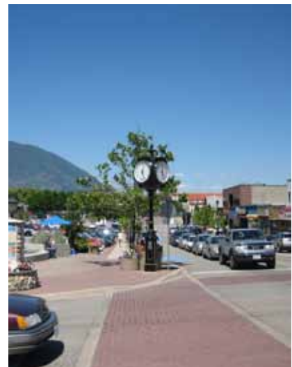
Paving denotes pedestrian crossing
