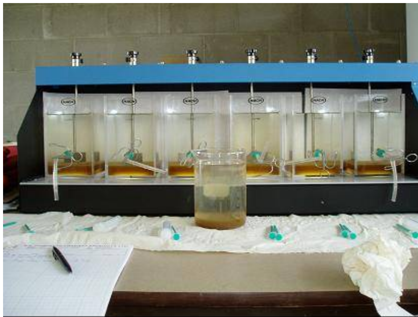
Figure A.11– Backwash water samples after 25 minutes of settling time (From the left; PACl 10, 25 and 40 mg/L, and 0, 25 and 40 mg/L of alum). Control test (with no chemical addition) was performed in the beaker shown.
