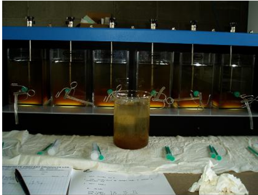
Figure A.10 – Backwash water samples after 15 minutes of settling time (From the left; PACl 10, 25 and 40 mg/L, and 0, 25 and 40 mg/L of alum). Control test (with no chemical addition) was performed in the beaker shown.
