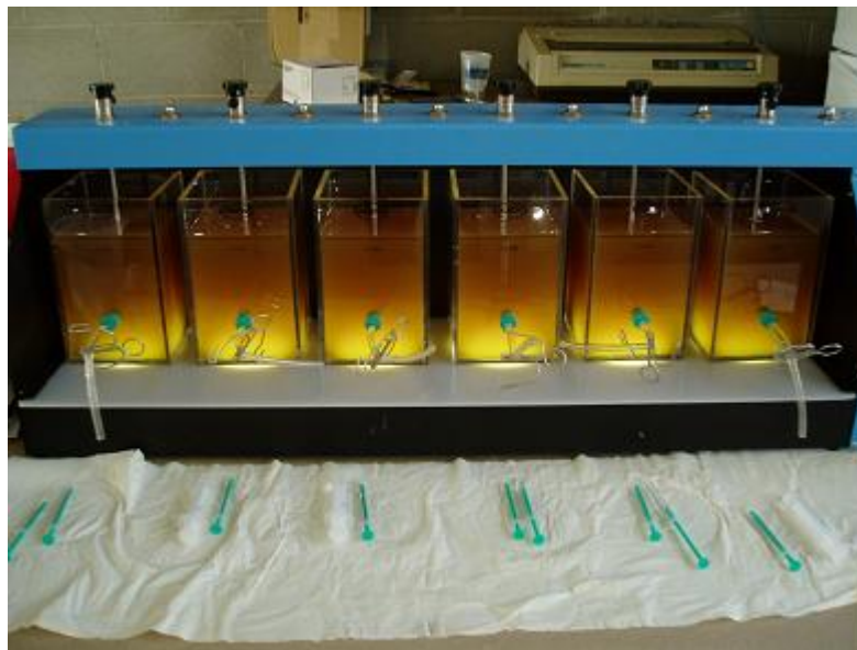
Figure A.9 – Backwash water samples at the start of the settleability tests.
