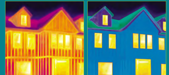
Figure 6 shows the results of “thermal imaging,” a tool for seeing where heat is being transferred through the building envelope. The top image reveals thermal bridges at every stud, as well as heat leaking around windows and through the roof. The lower image shows how an air barrier and continuous insulation has reduced thermal bridges and improved sealing around windows and doors.
