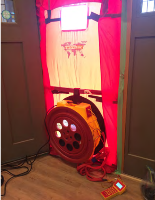
Figure 8: Blower door test in action
