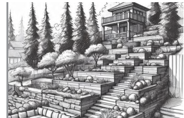
Stepped retaining walls
