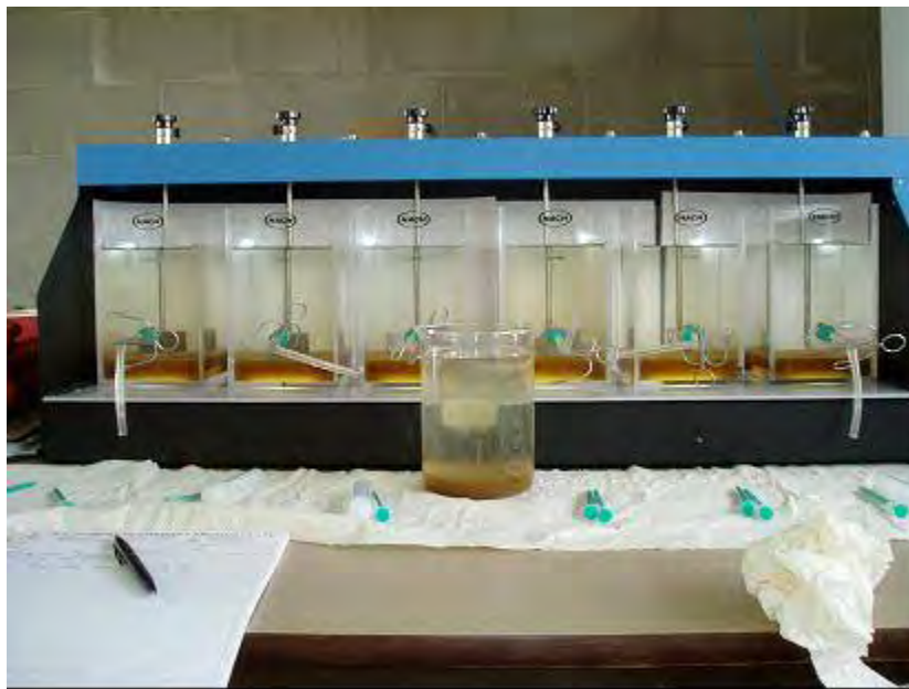
Figure A.11– Backwash water samples after 25 minutes of settling time (From the left; PACl 10, 25 and 40 mg/L, and 0, 25 and 40 mg/L of alum). Control test (with no chemical addition) was performed in the beaker shown.
