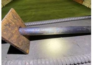
Photo 40: Typical bolt surface corrosion.
