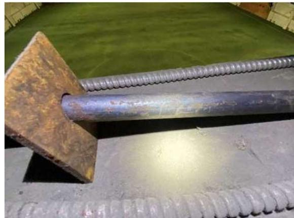
Photo 40: Typical bolt surface corrosion.
