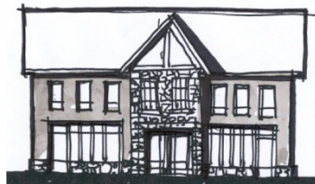
A good example of the use of material – the main entrance is accentuated with stone, the façade is limited to two primary materials, stucco and stone
