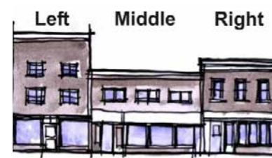
Left: a non-defined composition of the façade and poor proportions of the openings
