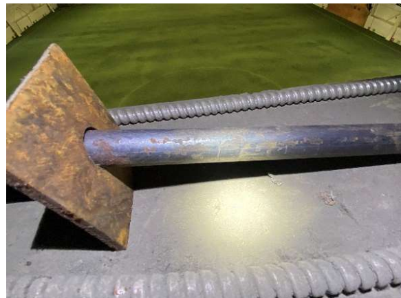
Photo 40: Typical bolt surface corrosion.
