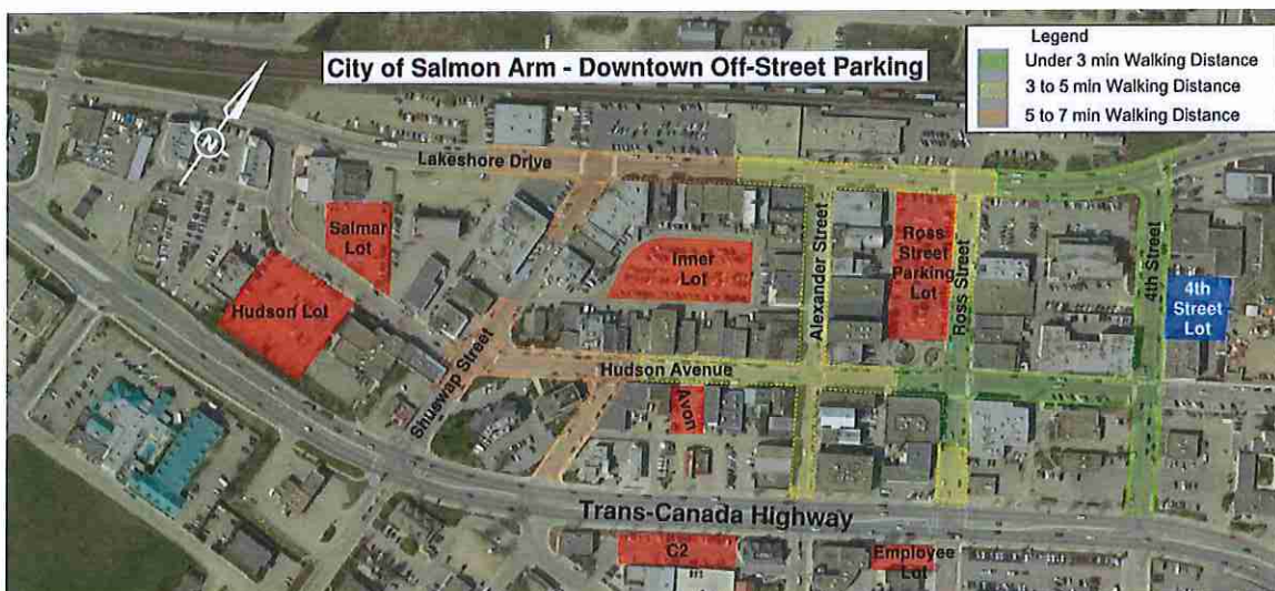
Figure ES.2: Estimated Pedestrian Walking Times from the Proposed Off-Street 4 th Street Lot using the Existing Sidewalk Network
