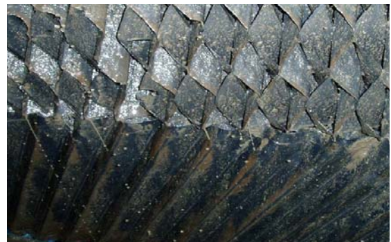
Cross Flow Media after sloughing
