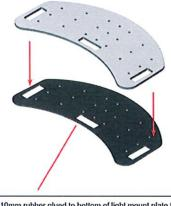
10mm rubber glued to bottom of light mount plate to prevent sliding/protect flat roof membrane
