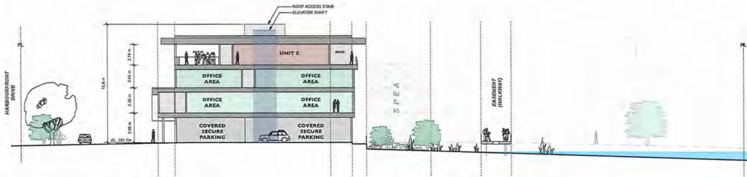
2 Building / Site Section Scale: 1:150
