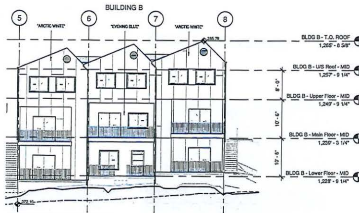
WEST ELEVATION - BUILDING B
