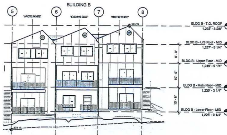
WEST ELEVATION - BUILDING B
