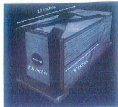
Marten box modified with fisher exclusion plate. The exclusion plate splits in middle and is held in place with thick rubber straps to allow of extraction of an animal.
