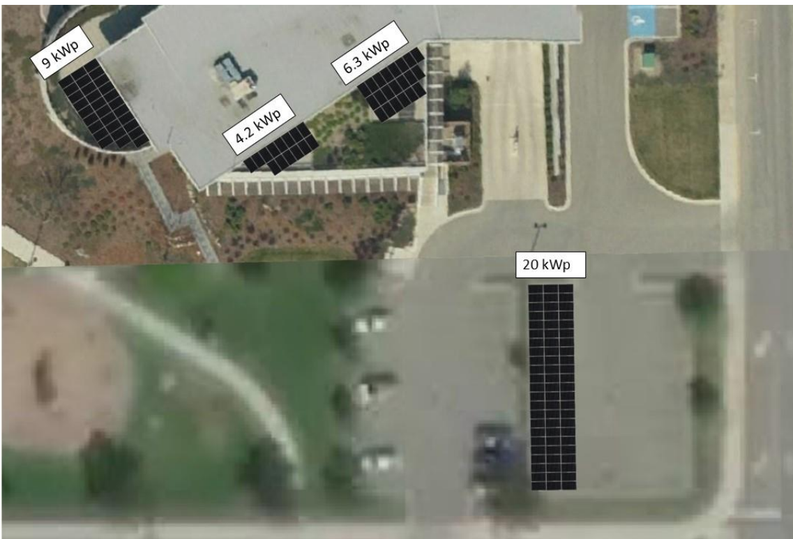
Figure 19: Example 19.5 kWp Solar Canopy and 20 kWp Parking Shelter Capacities
